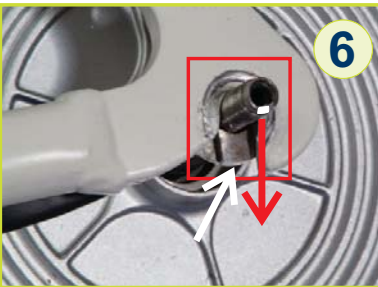
Insert wheel and make sure the blocker is engaged in the drop-out and that the nutch is pointing towards the ground.
