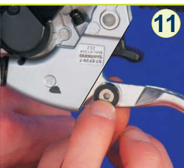
Clean underneath the brake lever with alcohol, acetone or brake cleaner and stick or screw magnet near the joint.
