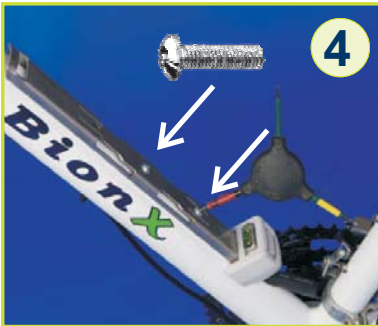
Screw battery slide. IMPORTANT: Please use screws included in BionX kit.
