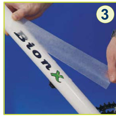
Put protective tape to avoid scratching the frame.
