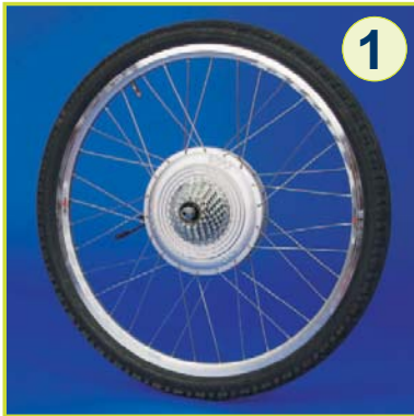
Mount tire + free wheel (8-speed max) on BionX rim.
