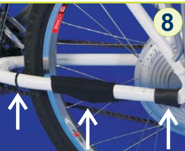
Connect, use tie-wraps and velcros to secure cabling.
