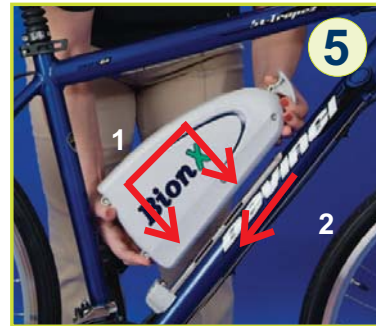
Put on frame and gently slide down towards the back.
