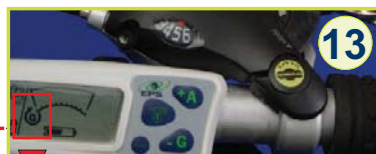
Please make sure the "G" comes on when you brake and goes away when you release the rear handbrake.
