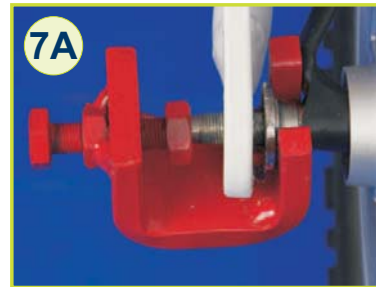
If the nutch is not pointing towards the ground, please use the puller (from BionX tool box) to free the blocker and then use a screw driver to adjust the nutch to the right angle.
