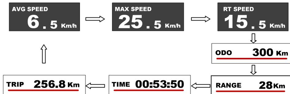
\*\*If there is no operation for 5 seconds, display will return Speed (Real-Time) display automatically.
