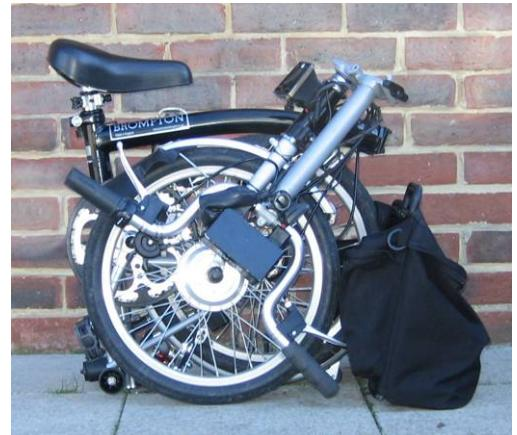
The Brompton–nano<sup>®</sup> is an electric bike kit specially designed for the Brompton folding bicycle. Using our small powerful nano<sup>®</sup> hub motor the Brompton–nano<sup>®</sup> gives the rider the extra assistance that takes out the effect of hills and headwinds, enabling you to arrive at your destination without the sweat!
