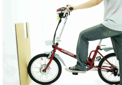
2. Then, press the main switch to either left (I) or right (II) position while depressing the pedal.
