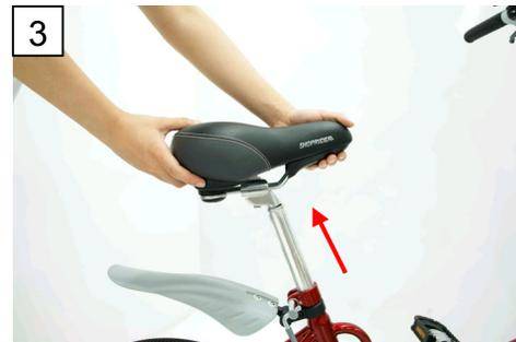
Loosen the clamp lever to remove the saddle.
