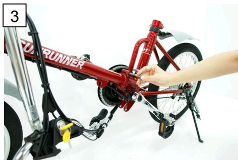
3 Coincide the locking holes and insert the safety pin to engage the front and rear frame assembly securely.
