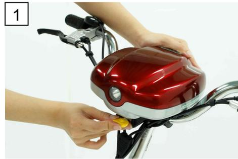
Refer to the instruction for Dismounting Battery Case to remove the battery case.
