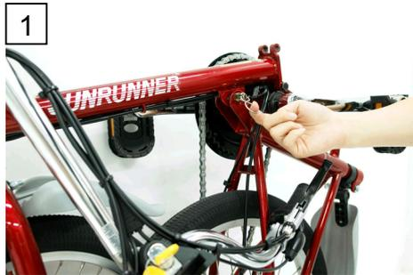
1 Remove the safety pin from the locking hole.
