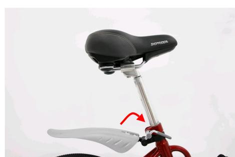
4. Tighten the clamp lever.
