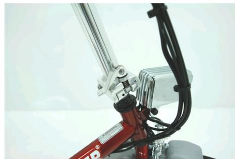
4 Lower the lever by fingers as shown to retreat the pin for the engagement of the handle bar. Restore the handle bar and then heighten the lever to engage pin and slot in, and then clamp the lever to secure the handle bar.
