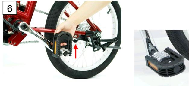
Pull the trigger of the pedal and unfold the pedal simultaneously. Repeat the same steps on the other side of the pedal.
