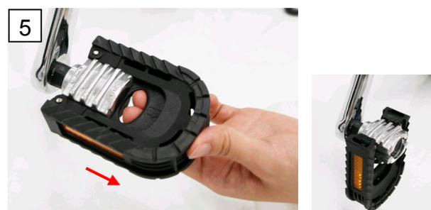
Pull the trigger of the pedal and fold the pedal simultaneously. Repeat the same steps for the other side of the pedal.
