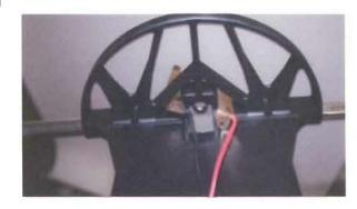
Secure ends of copper connectors into the slots on either side of the plastic frame as shown. Stretch the connectors so that they are tight against the inside of the plastic moulding. It is useful to secure them in place by sliding in the brompton luggage block whilst securing them in place.
