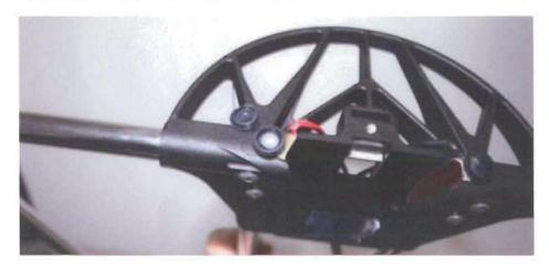
Make a hole in the rear face of the inside of the Brompton bag half way up. Feed the battery cable through and refit the bag frame.
